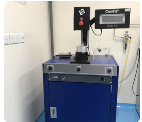
TSI Automated Filter Tester Model 8210 for penetration test
