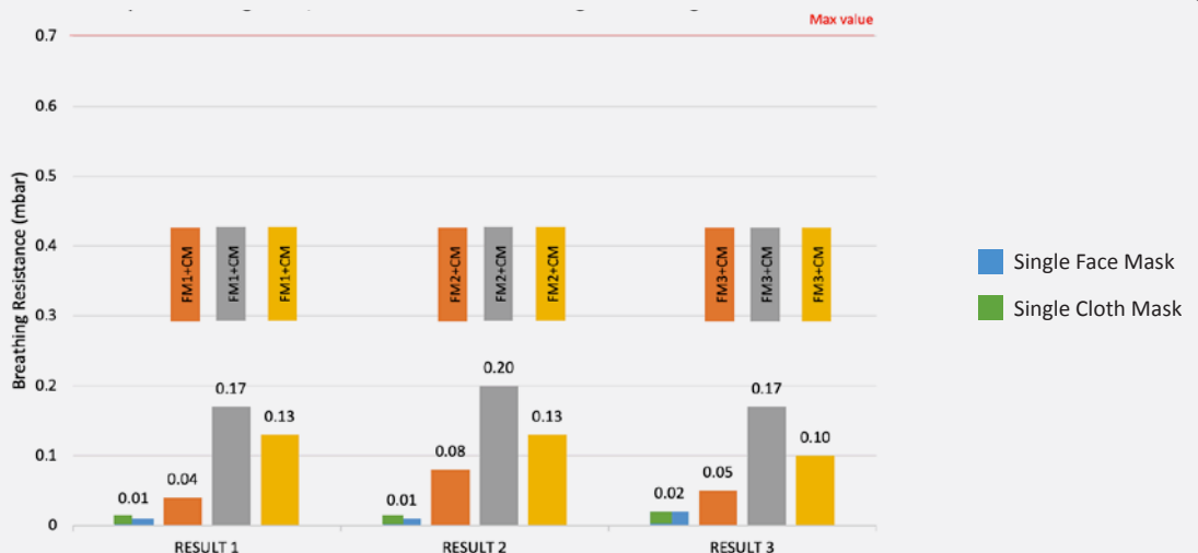
Figure 2: Comparison of single face / cloth mask and double-masking on breathing resistance
