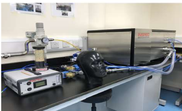
Carbon dioxide rig – carbon dioxide analyser, breathing machine and dummy head
