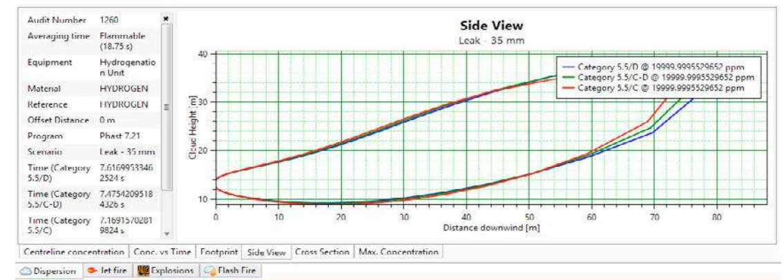
Figure 6: Side View of Hydrogen Cloud vs Downwind distance at 35 mm Leak
