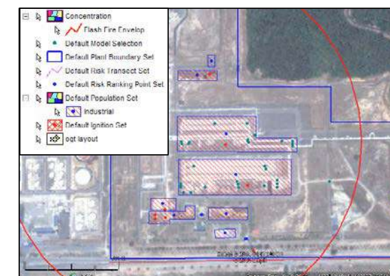
Figure 4: Initial Worst Case for Flash Fire Result (501 meter)
