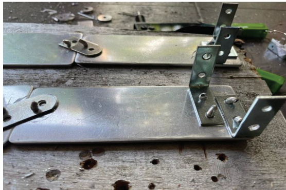
Figure 2.2: The Fitting Task of Shaped Aluminum Sheet Using a Bracket and a Rivet
