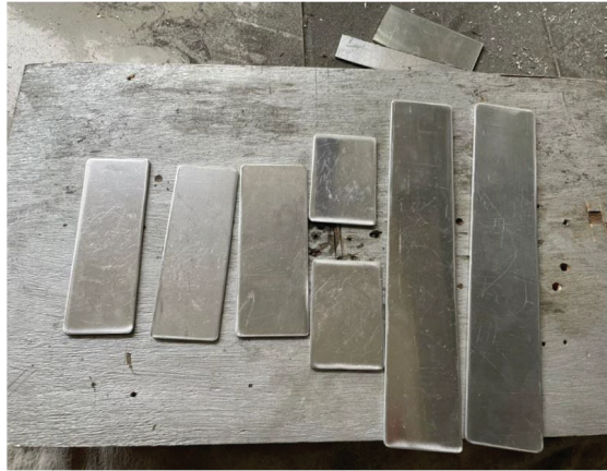
Figure 2.1: The Result of an Aluminum Sheet After Being Shaped Using Grinder During Fabrication
