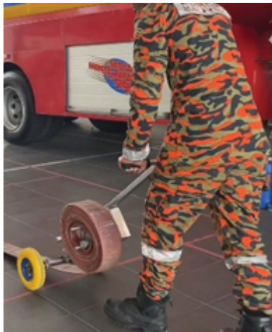
Figure 2.4: The Testing Process of Hose Roller at Pagoh Fire Station
